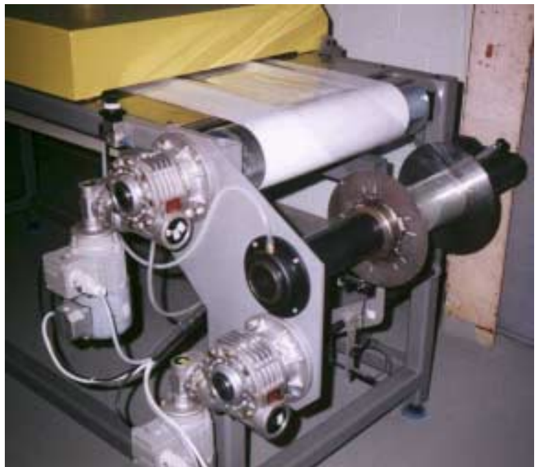
Heating station. The heating plate is holding on open position by gas springs.
