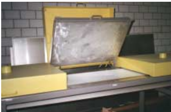
Heating station. The heating plate is holding on open position by gas springs.
